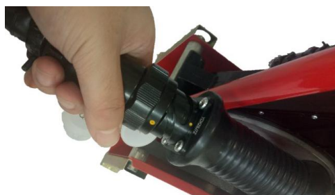
Connection between the cable and heating plate
