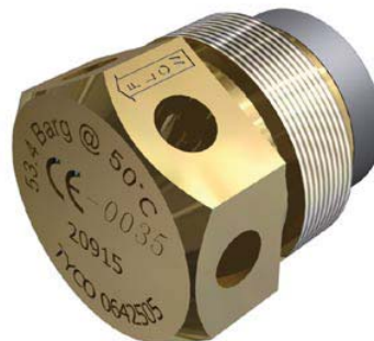
Burst Disc for 25 mm (1") Valve Part No. 20915
